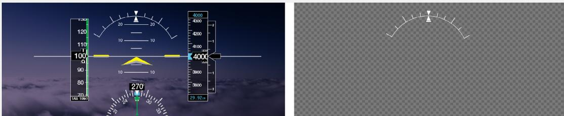
The image **bank\_angle.png** shown on the right uses dimensions that match the display size of the cockpit application which unnecessarily uses large areas of full transparency which results in a negative impact on performance.
